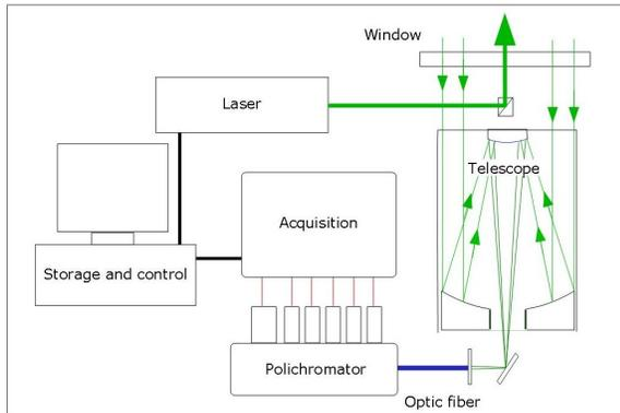
Figure 2. block diagram of the lidar system.
