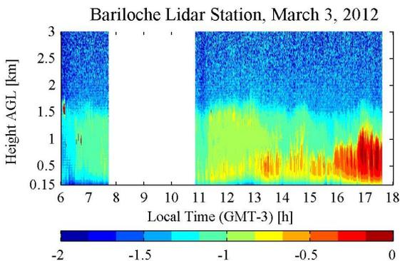
Figure 4. Lidar backscatter profiles at 1064 nm (6 s averaging time, 7.5 m spatial resolution) with volcanic ashes on March 3.
